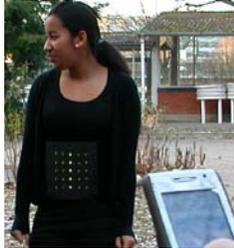
Figure 5. LED-array on shirt
