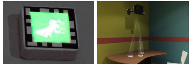
Figure 6. Projection on block with frame marker and setting for using ARBlocks
