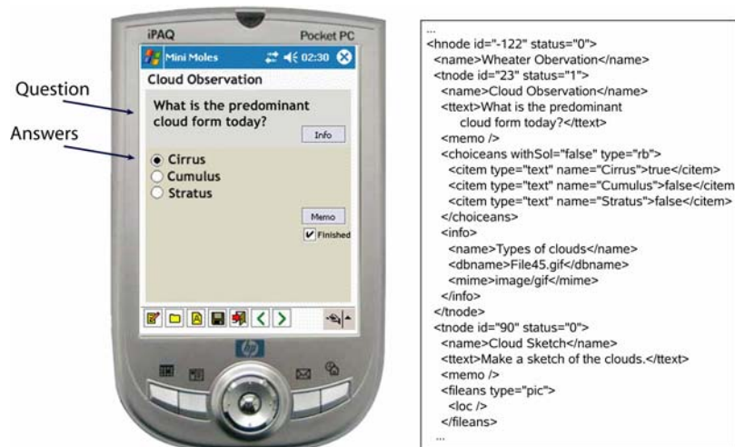
Figure 3. Mini Moles questionnaire on a PDA: a multiple choice question ( left 1 ) and respective XML file extract ( right )
