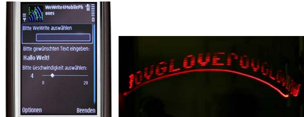
Figure 7. Interface of WeWrite and long-exposure picture of the glove-mounted LED array
