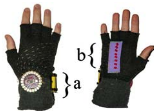
Figure 6. Glove with a) LilyPad, upper side and b) LED-column on the reverse side
