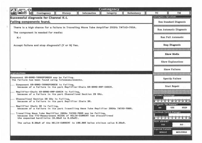
After a failure has been found, REPLEX is able to explain the inference path that led to the diagnosis (cf. Fig. 2). This improves the system's transparency and gives the user deeper insight into repeater-equipment dependencies.
