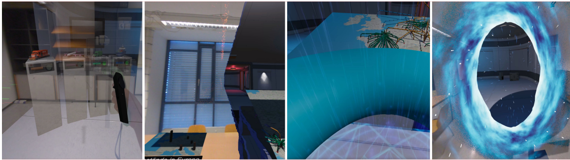
Figure 1: Four transition techniques from the user's perspective during the transition between augmented and virtual reality in the context of data visualisation. From left to right, Fade , SimpleCut , TeleportBeam and Portal .
