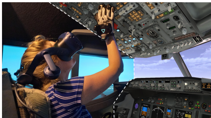
Fig. 1. Our study compared a full-scale physical cockpit of a Boeing 737-800NG that was part of a flight simulator (left) to an exact replica in a virtual reality flight simulator including visual, auditive, and vibrotactile feedback (right) to understand how well current virtual reality technologies can simulate such safety-critical interactive spaces with many physical controls.
