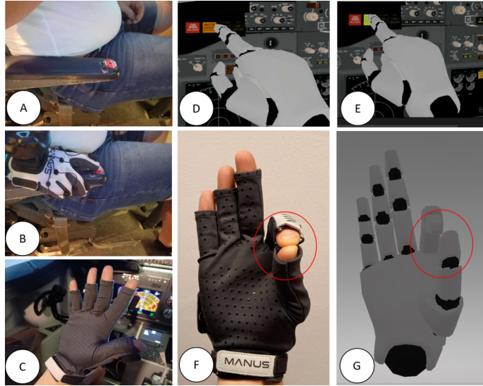
Fig. 2. Details of our study: (A) tangible marker at starting position on right armrest (red), (B) participant puts right index finger at starting position, (C) no fingertips were covered by the gloves to enable unimpaired physical interaction with real cockpit switches in PFS, (D) and (E) visual feedback when touching a control in VR. (F) and (G) slight mismatch between physical hand and hand representation in VR when touching the finger tips of the index finger and the thumb.
