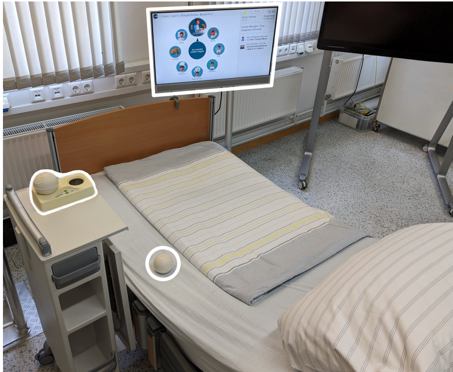
Fig 8: Laboratory setup of the evaluation. The central components are highlighted: the ball-shaped interaction device on the bed, its charging station on the bedside table, and the mounted display at the foot of the bed.
